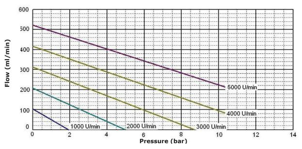
Performance curve based on: medium water, temperature 20°C, viscosity 1 cP, bypass closed
